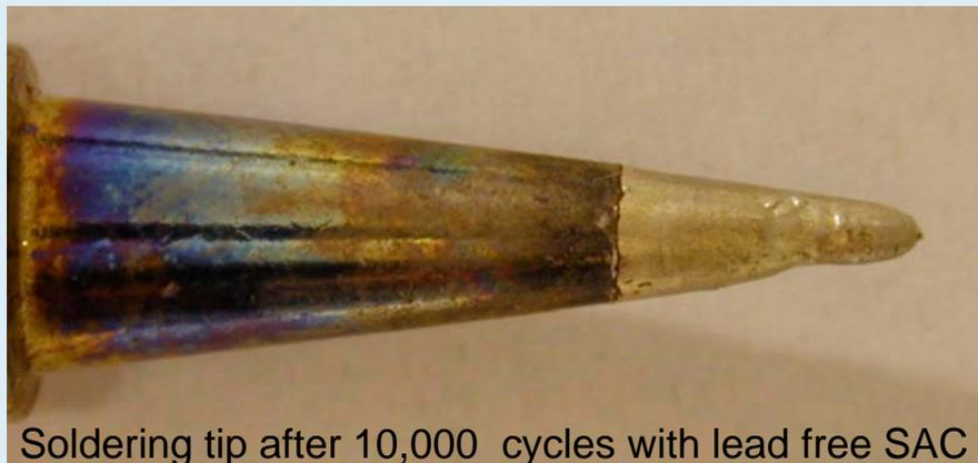
Soldering tip after 10,000 cycles with lead free SAC
