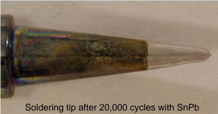
Soldering tip after 20,000 cycles with SnPb
