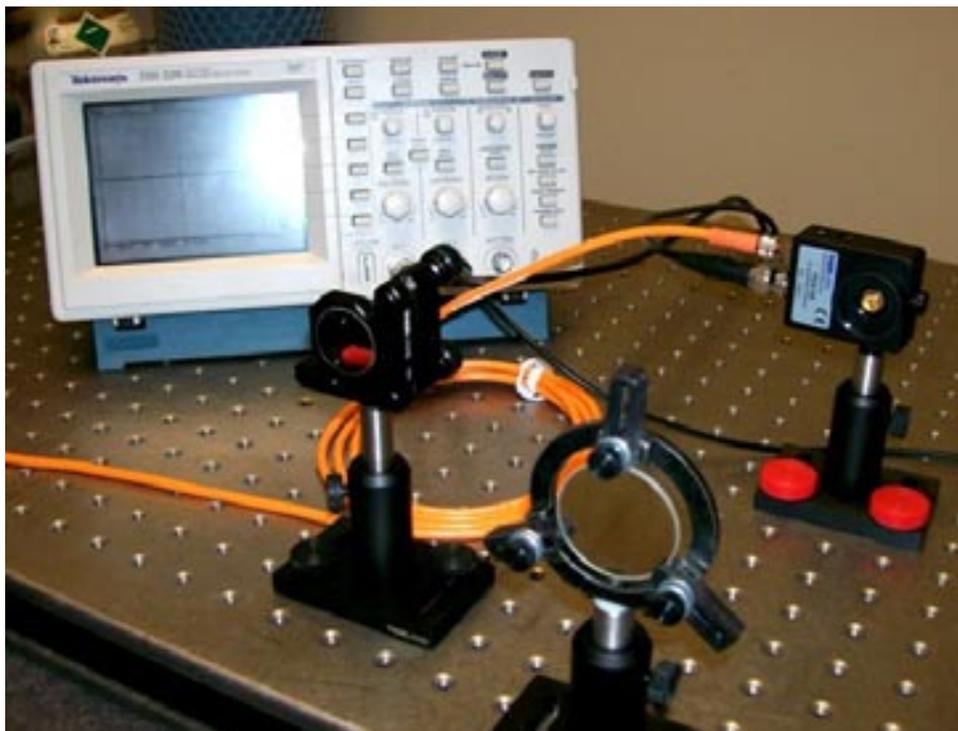
The detector arrangement, with focusing lens.
