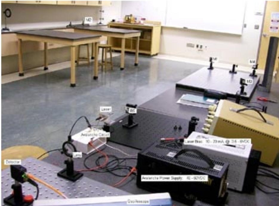
The overall setup showing mirrors, laser, drive circuit and detection circuit. The pulse delay measured corresponds to the optical path delay between the two paths:
